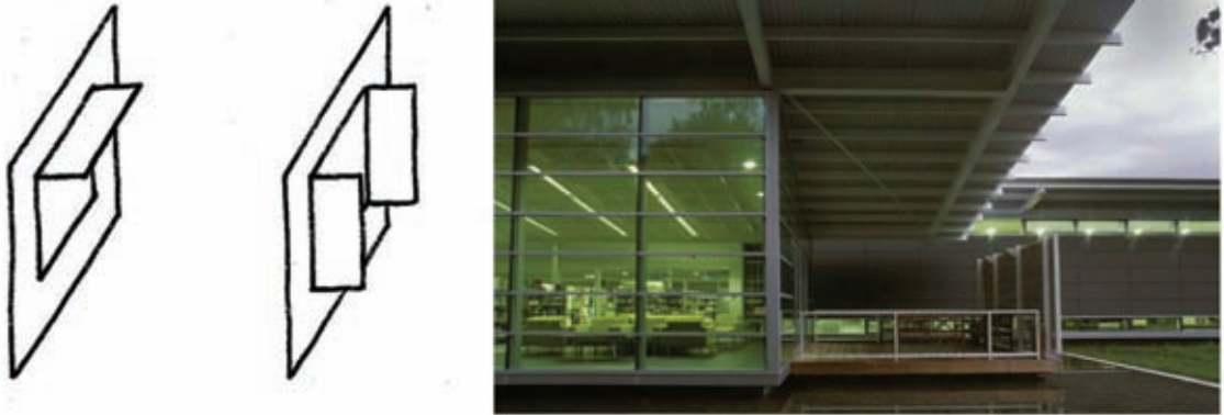
Figure 7: Overhangs (left) and sidefins (centre)
